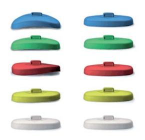
NC 00607 PP diminishes the effect that pigments have on the shrinkage of injection molded articles. Left side without NC 00607 PP and right side with NC 00607 PP.
